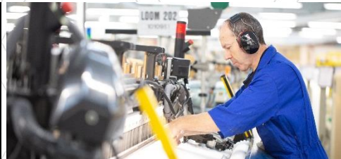
Setting up one of the high-speed looms for DecelAir Superlight fabric
