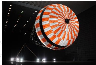
A parachute made with Heathcoat's fabric is tested at NASA Ames Research Centre
